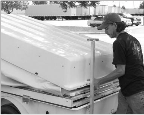
8. Lower roof from top of telescopic poles.
